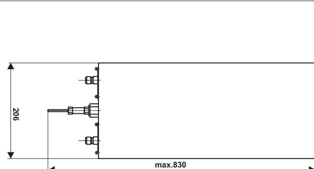
Bandpass filter BPC161.206 is one quarter wavelength cavity resonator. This filter can be used a preselector to protect a receiver, or it can be used to reduce spurious output from a transmitter, or can be used in special duplexers.
