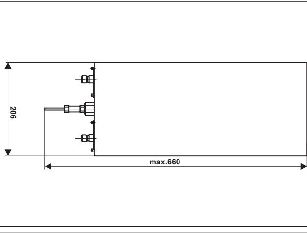
Bandpass filter BPC201.206 is one quarter wavelength cavity resonator. This filter can be used a preselector to protect a receiver, or it can be used to reduce spurious output from a transmitter, or can be used in special duplexers.
