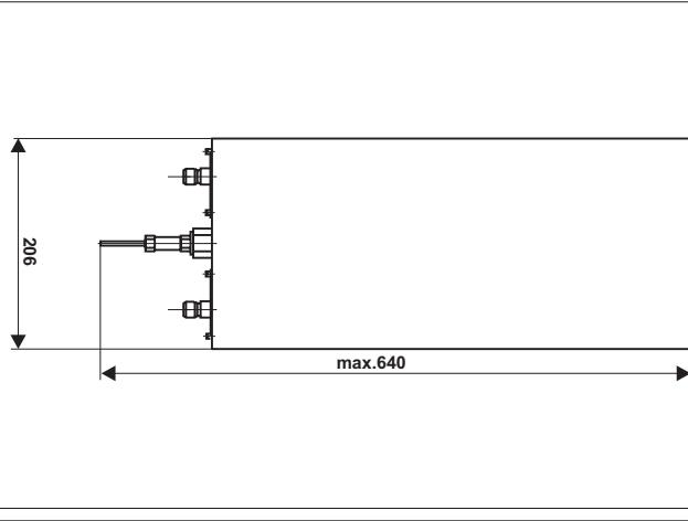
Bandpass filter BPC251.206 is one quarter wavelength cavity resonator. This filter can be used a preselector to protect a receiver, or it can be used to reduce spurious output from a transmitter, or can be used in special duplexers.
