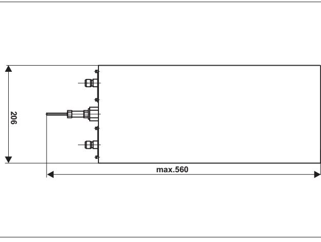
Bandpass filter BPC301.206 is one quarter wavelength cavity resonator. This filter can be used a preselector to protect a receiver, or it can be used to reduce spurious output from a transmitter, or can be used in special duplexers.
