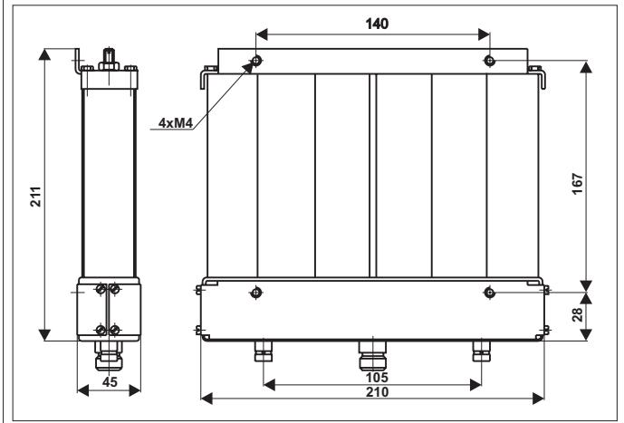
The helical duplexer HDF406.Q34 is a symmetrical duplexer made of six full-length  $1/4 \lambda$  resonators in a Band-reject configuration. The duplexer is designed for the operation of the transmitter and receiver together in to one antenna in bands of 400-440 MHz.
