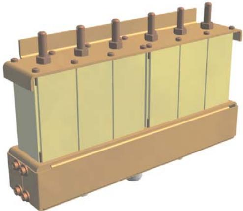
The helical duplexer HDF386.Q34 is a symmetrical duplexer made of six High Q helical resonators in a Band-reject configuration. The duplexer is designed for the operation of the transmitter and receiver together in to one antenna in bands of 380-430 MHz.
