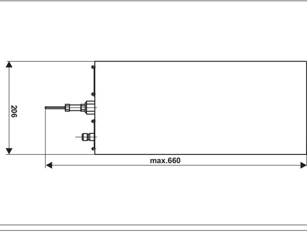
S-P filter (Stop-Pass filter) SPC201.206 is one quarter wavelength cavity resonator. This filter can be used in the transmission path to suppress side band noise and to attenuate intermodulation products at the receiving frequencies, in the receiving path to attenuate transmitting frequencies or as a component for antenna combiners with very low frequency spacing.
