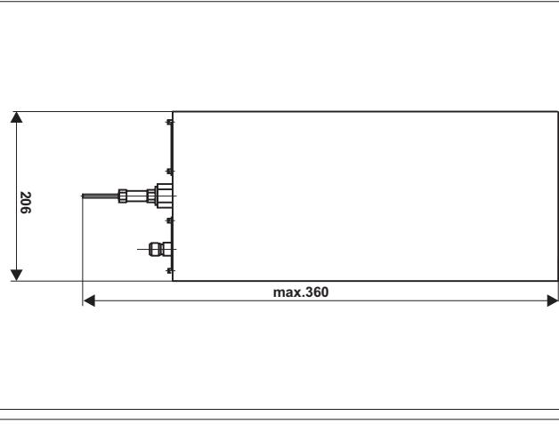
S-P filter (Stop-Pass filter) SPC501.206 is one quarter wavelength cavity resonator. This filter can be used in the transmission path to suppress side band noise and to attenuate intermodulation products at the receiving frequencies, in the receiving path to attenuate transmitting frequencies or as a component for antenna combiners with very low frequency spacing.
